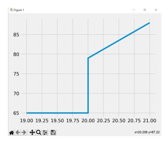
I also used the animation library which allows for a live graph with new input updating the live graph. I opened a CSV file which was being written and read from another script and inputting the data from the CSV file to the graph.
